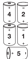
Insert the batteries in the dispenser. Pay attention to correct polarity and sequens as above!
