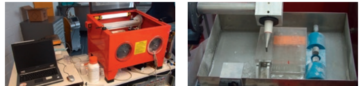
Fig. 1: Test setup of Air Box Test with PC control to the left, jet tub with sample holder and adjustable jet nozzle to the right.
